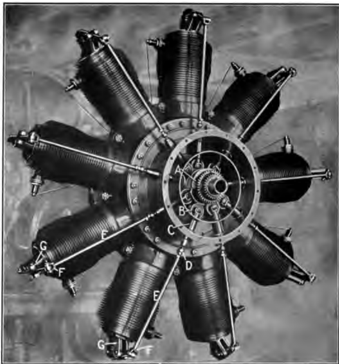
FIG. 88.—Cam action of Gnome engine.
